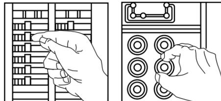
Next, plug in and turn ON the lamp or radio at the receptacle's other outlet to make sure the power is OFF at both outlets. If the power is not OFF, stop work and call an electrician to complete the installation.
