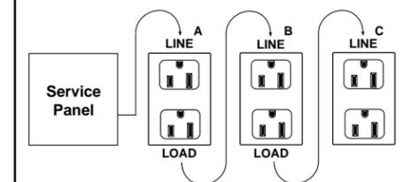
Placing the GFCI in position A will also provide protection to "load side" receptacles B and C. On the other hand, placing the GFCI in position C will not provide protection to receptacles A or B. Remember that receptacles A, B, and C can be in different rooms.
